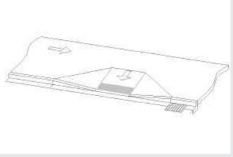
determines the cross slope of perpendicular ramps and landings at mid-block crossings. Exceptions are provided for ramps located at mid-block crossings that permit the cross slope of the ramp and landing to be greater than 1:48 so that the ramp can transition smoothly to the street crossing. Otherwise, maintaining a 1:48 cross slope at streets with a steeper grade would result in a warped transition from the ramp to the road, which is problematic for wheelchair maneuvering.
